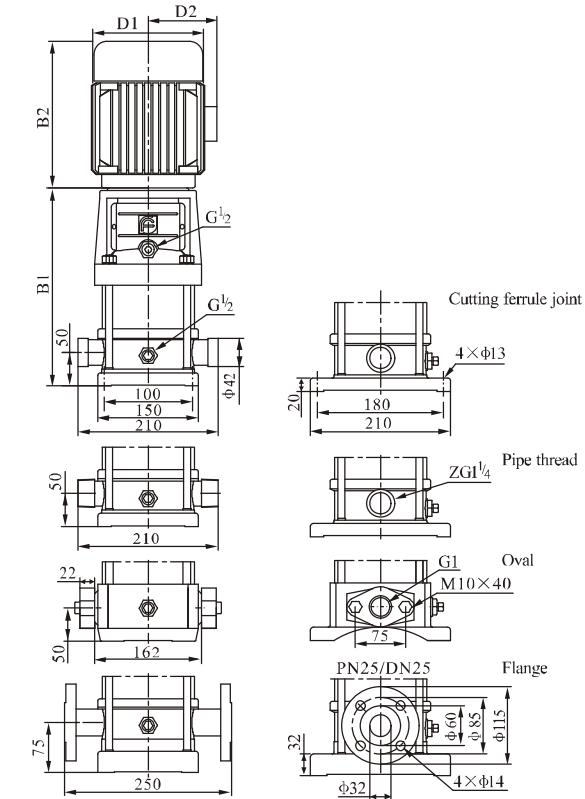
CDL3-25 ~ 3-36 sub-connection of pipeline has no oval flange connection.
