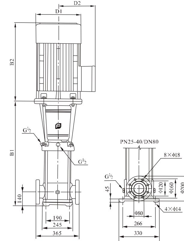
The overall dimensions of explosion-proof motor is a little different. Pls contact us for details.
